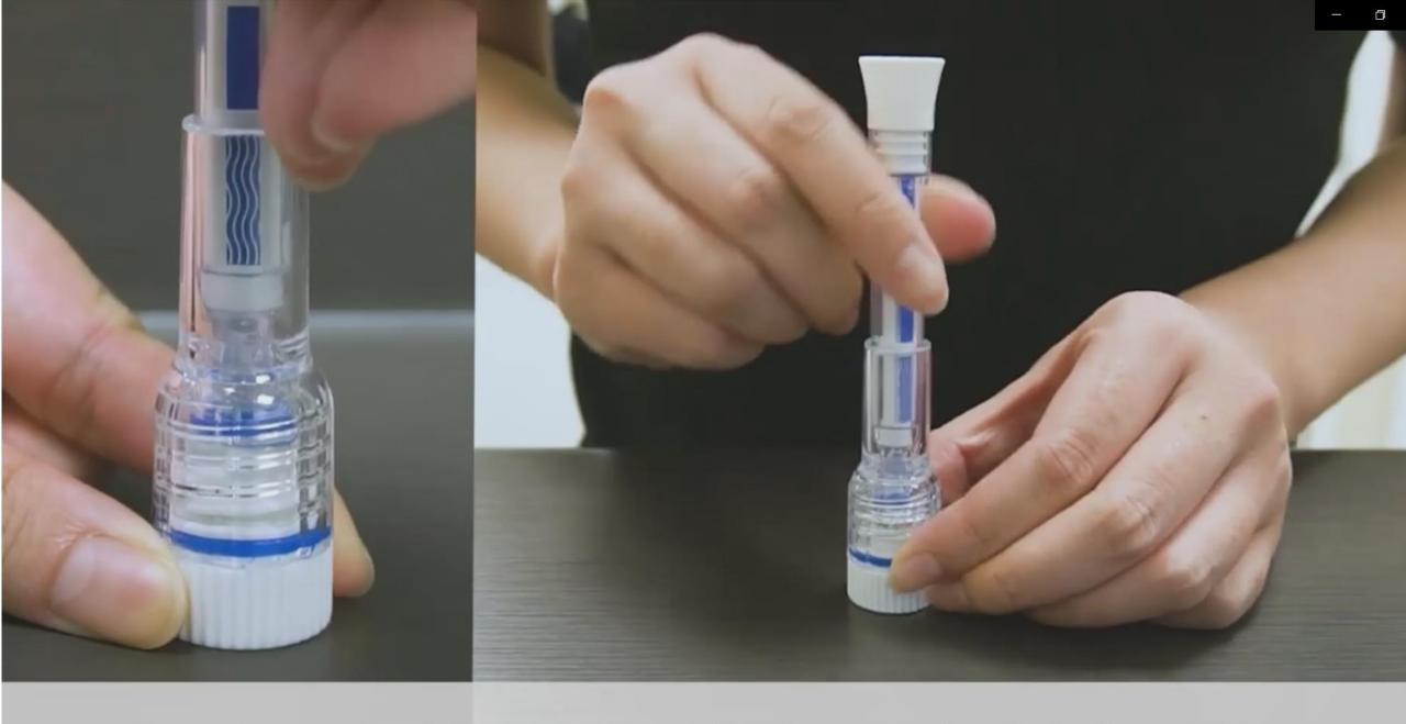
Press down to break the seal of the Buffer Cap, releasing the buffer solution.
